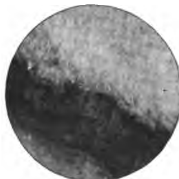
Fig. 32. Crack between Carburized Shell and Core
